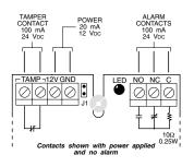
NOTE: This unit is UL Listed and should be connected to a listed control unit or power supply providing at least 4 hours of standby power.
